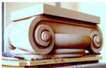
The Gillingwater half-capital reconstruction carved out of stone and based on measurements taken from the pilaster capital on the left.
